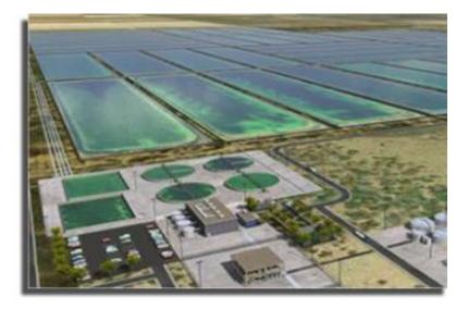
To make a biorefinery more cost effective and sustainable, waste sources of heat, CO<sub>2</sub> and nutrients that can be found from power plants, factories, and water treatment plants would be used as the nutrients for the algae. This model has been recently adapted by companies such as Sapphire energy. Still, there are problems that can only be solved by further research.
